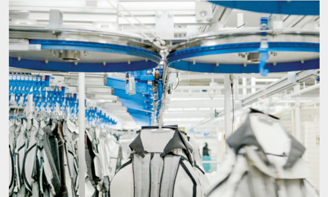
Dynamic storage: Filtering and transporting the required covers to the sorter unit
