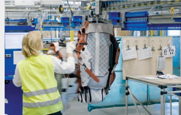
Incoming Goods: Attachment to clamps, scanning and automatic loading of the seat covers
